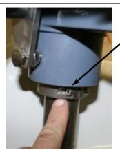
Step 3: Loosen and lower post holding collar
