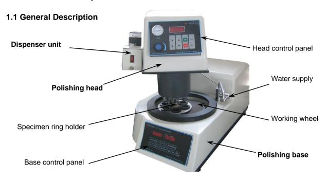
The GP 1000A is a variable speed polishing head (0-200 rpm) for use with the grinding/ polishing base machine for automated metallographic specimen preparation. It can also run either automatically with the polishing base or in a manual mode with independent control.
