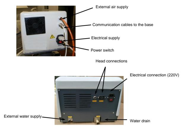
External air supply: It is recommended that the air supply be clean, filtered and lubricated to extend the life and
