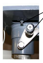
Rotate lever to disengage button
