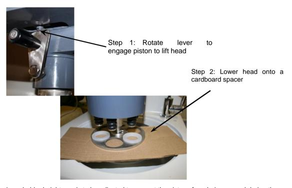
The specimen holder height needs to be adjusted to prevent the pistons from being ground during the operation of the machine.
