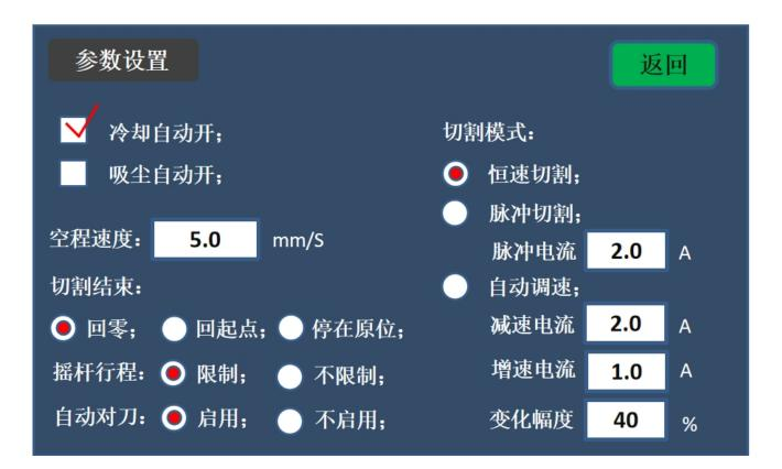
Automatic cooling on: it is on by default. In automatic mode, one key start and one key cutting can be realized.
