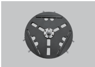
Side locking fixture Sample holder diameter: 160mm or 180mm Maximum sample size: 50x30mm Maximum sample height: 5mm 25.03.830 610-103 25.03.840 610-104
