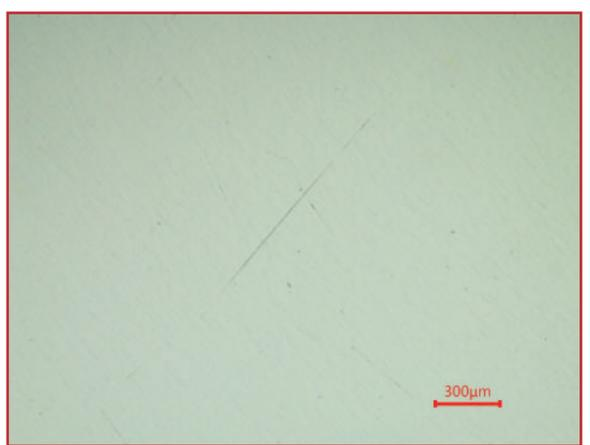
Specimen polished with ZN-ZP cloth and 50nm colloidal silica suspension– 50X
