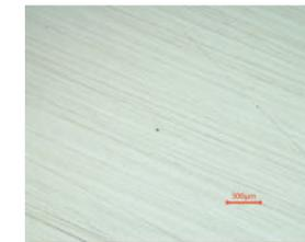
POS disc with 9µm Diamond Polishing Suspension for 3 minutes
