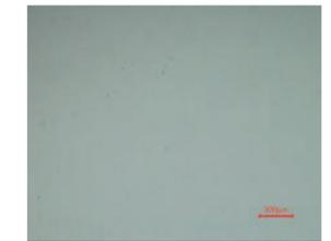
SC-JP Polishing Cloth with PD-WT 3µm Polycrystalline Diamond Polishing Suspension for 3 minutes
