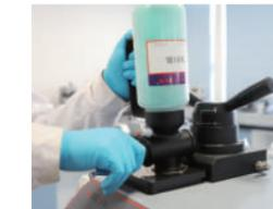
Application: Quantitative addition of hot mounting resin to prevent dust contamination in the air.
